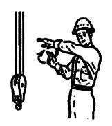
MOVE SLOWLY. Use one hand to give any motion signal and place other hand motionless above the hand giving the motion signal. (Hoist slowly shown as example.)
