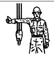
RAISE BOOM. Extend arm, fingers closed, thumb pointing upward.
