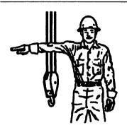
SWING. Extend arm, point with finger in direction of swing of boom.
