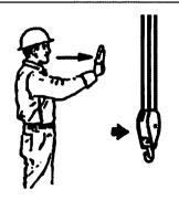
TRAVEL. Extend arm forward, hand open and slightly raised; make pushing motion in direction of travel.
