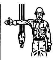
RAISE THE BOOM AND LOWER THE LOAD. With arm extended, thumb pointing up, flex fingers in and out as lone as load movement is desired.
