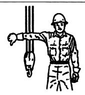
LOWER BOOM. Extend arm, fingers closed, thumb pointing downward.
